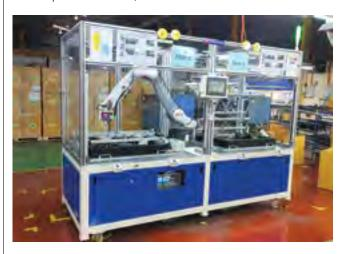
Automated Drilling Machine for Suspension Division which significantly improved efficiency and accuracy while reducing reliance on manpower.
