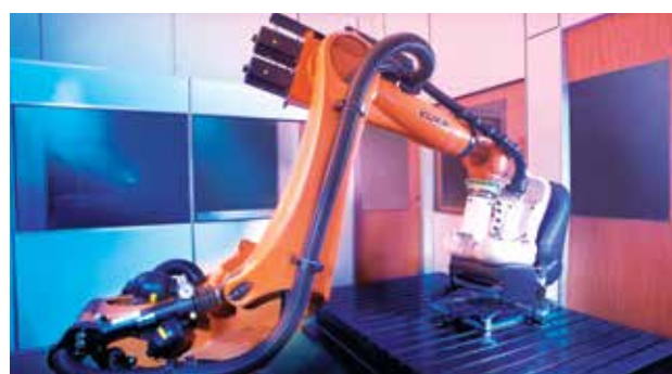
Ingress and egress machine
