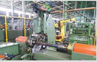
Fully Automated NC Coiling Machine with Robotics Transfer
